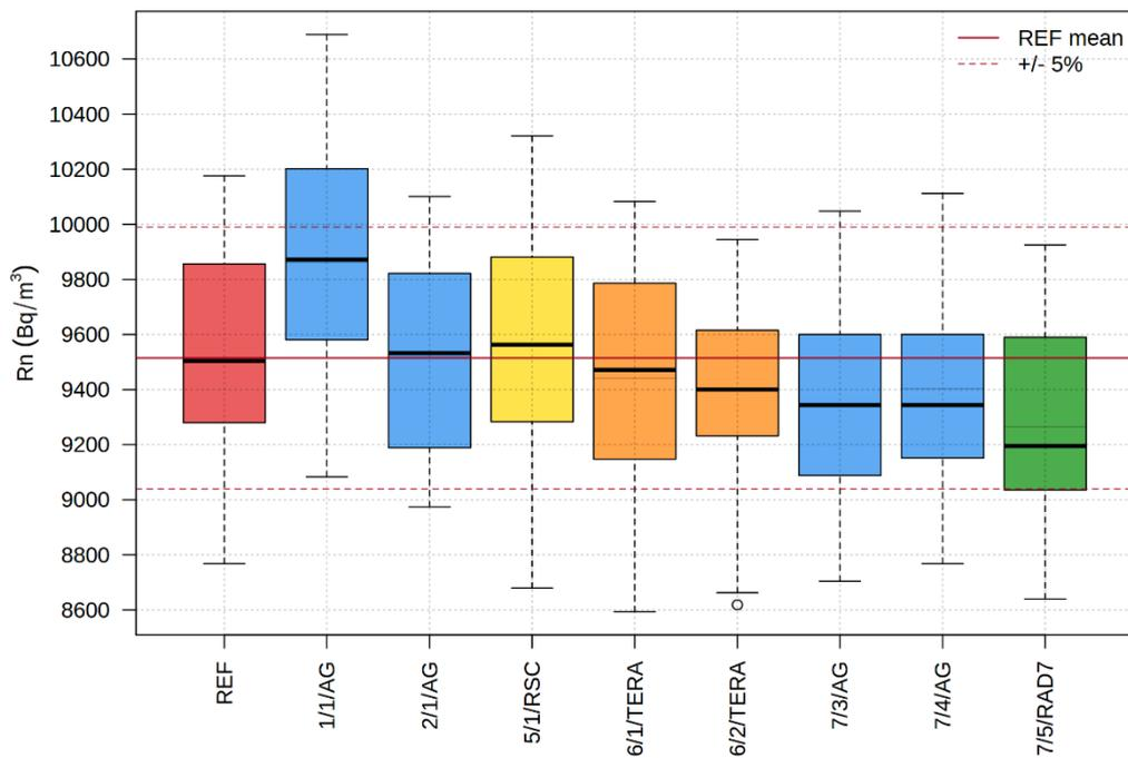
Fig. 8 Boxplot representing data from continuous monitors during A<sub>2</sub>. Top panel show all monitors, the bottom panel shows the same data without five outlying monitors. Colours represent different types of monitors.
