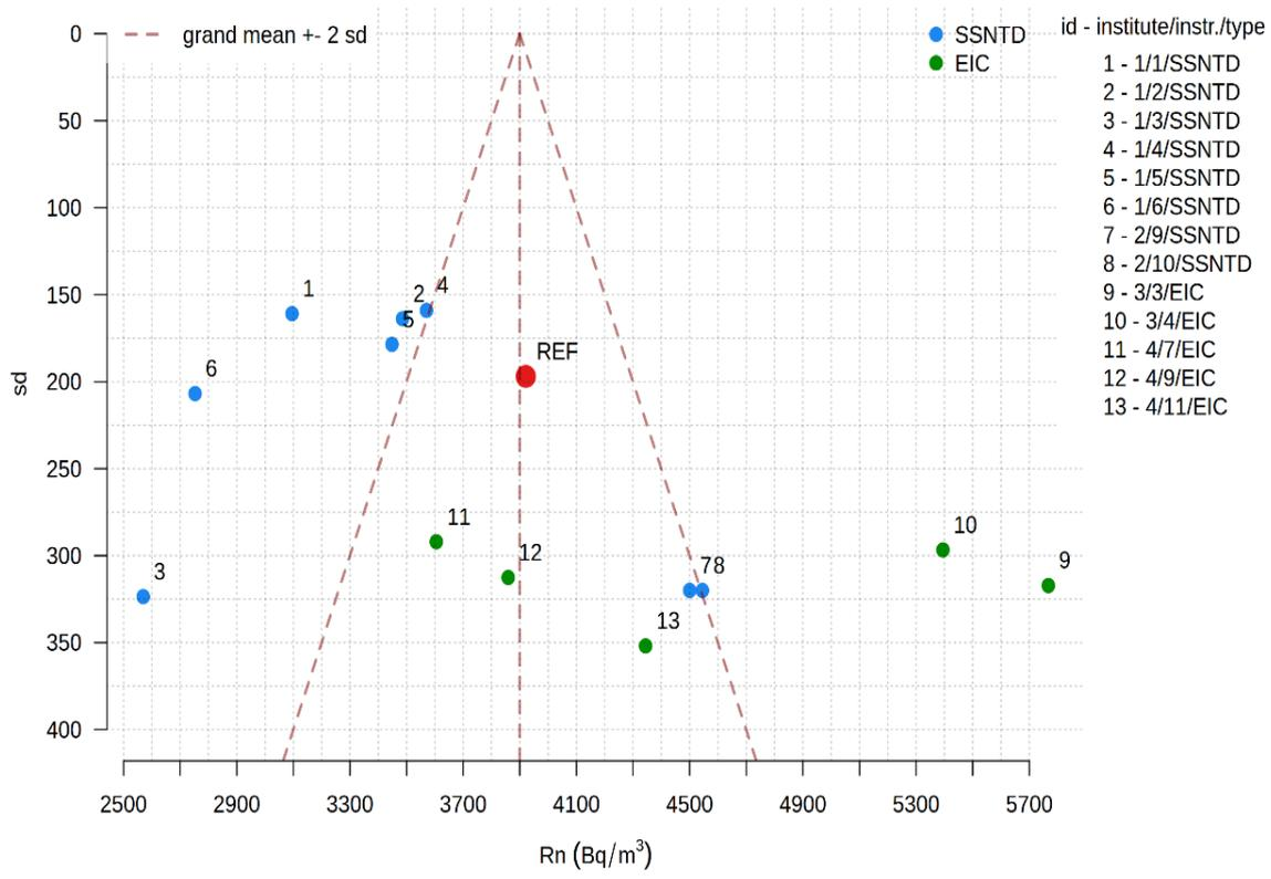
Fig. 15 Results for radon integral systems during B<sub>2</sub>. Top panel - forest plot. Red lines represent the reference mean together with ± 5%, 20%. Bottom panel – funnel plot.
