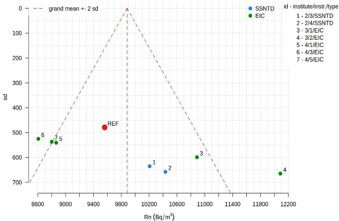
Fig. 12. Results for radon integral systems during B<sub>1</sub>. Top panel - forest plot. Red lines represent the reference mean together with ±5%, 20%. Bottom panel – funnel plot.
