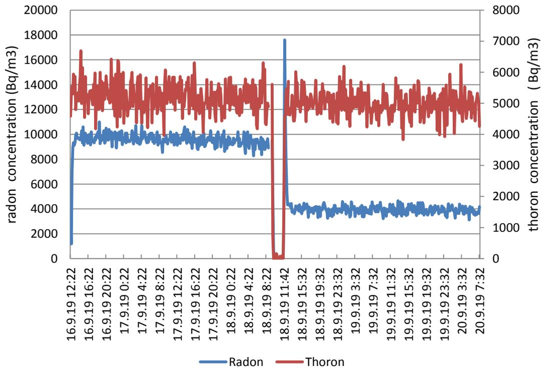
Fig.2 Time variations of radon and thoron concentration from the beginning of  $B_1$  to the end of  $B_2$  exposure.
