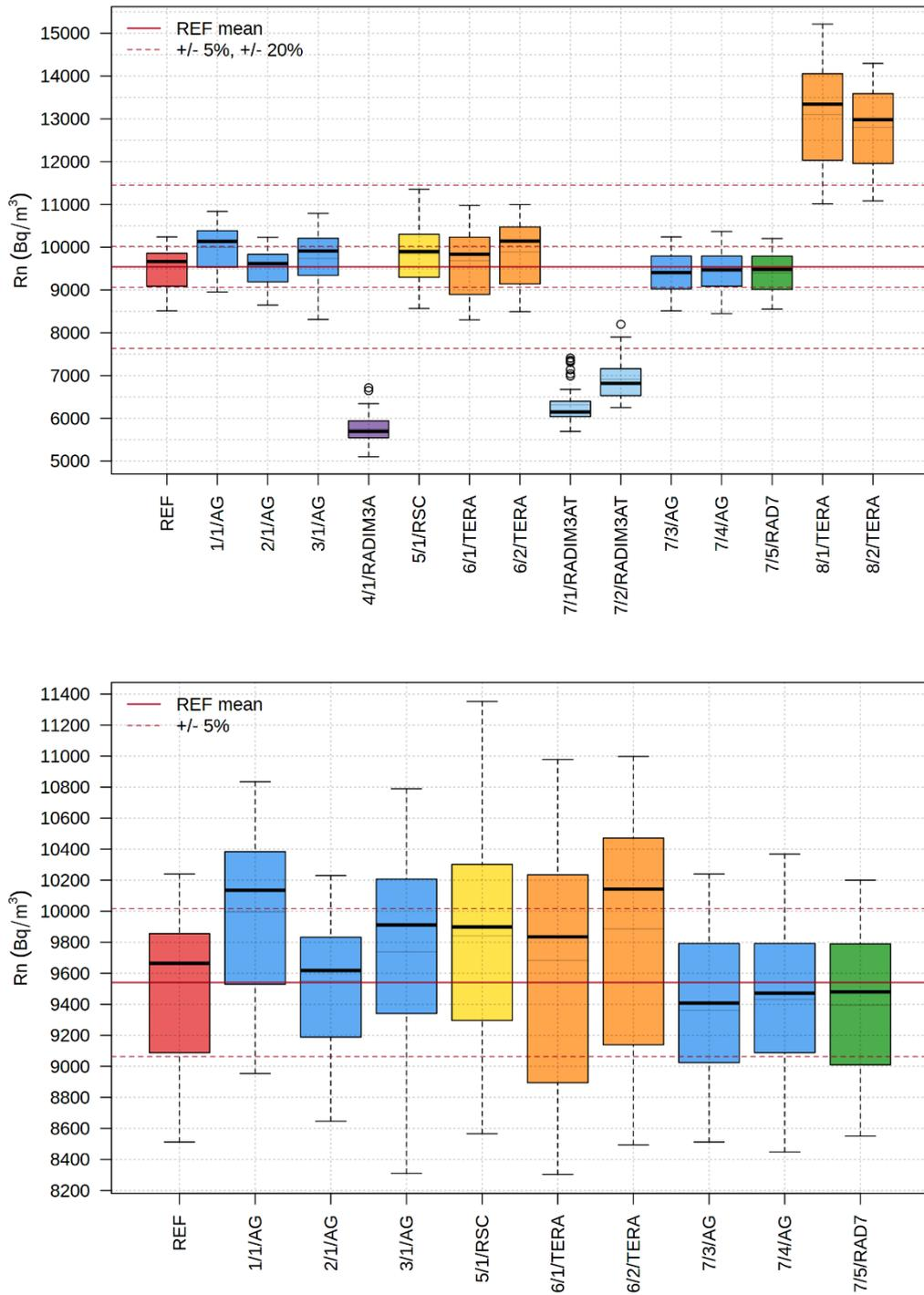
Fig. 5 Boxplot representing data from continuous monitors for  $A_1$ . Top panel shows all monitors, the bottom panel shows the same without five outlying monitors. Colours represent different types of monitors.
