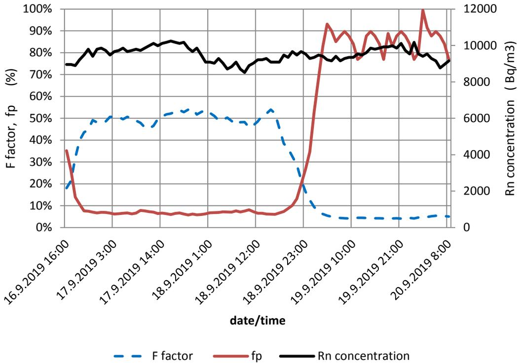
Fig.1 Time variation of radon concentration, equilibrium factor F and  $f_p$  from the beginning of  $A_1$  to the end of  $A_2$  exposure
