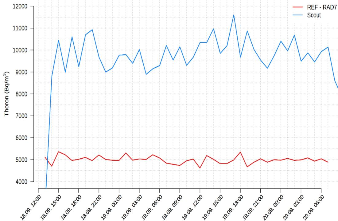
Fig. 14 Radon (top panel) and thoron (bottom panel) concentration during B<sub>2</sub> for the reference RAD7 monitor and the participant's Scout monitor.
