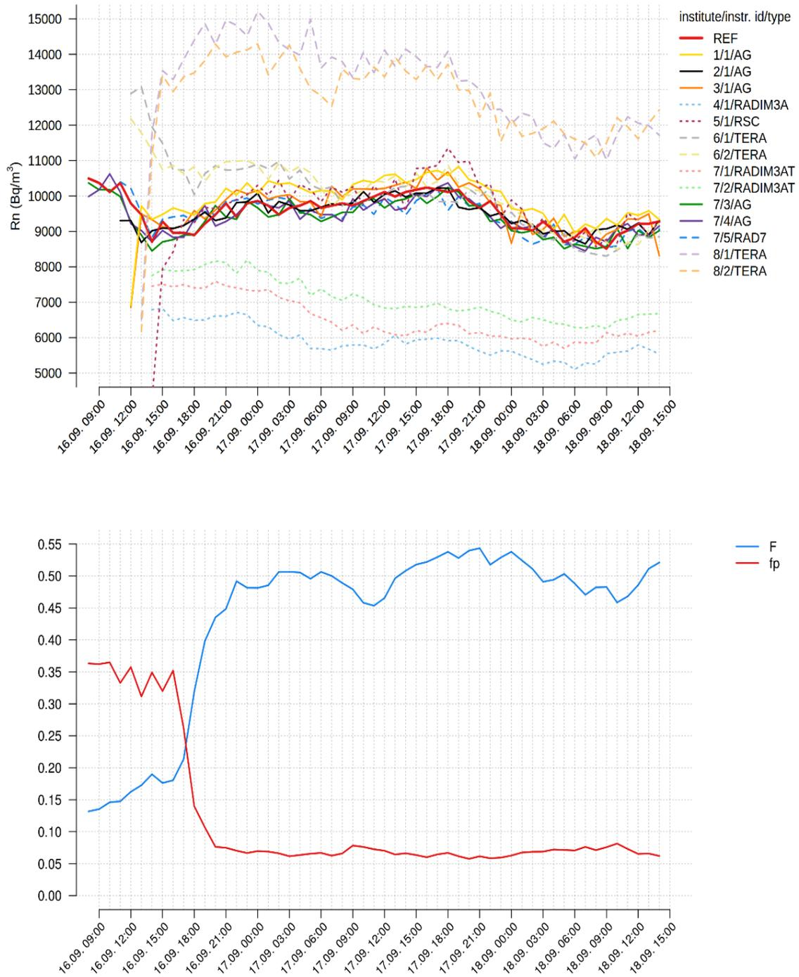
Fig. 3 Top panel – data from all radon continuous monitors during A<sub>1</sub>. Bottom panel – factor F and f<sub>p</sub> during A<sub>1</sub>. Note that not all the data that are shown in the figures are not used for the analysis.
