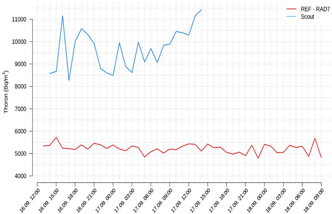
Fig. 11 Radon (top panel) and thoron (bottom panel) concentration during B<sub>1</sub> for the reference RAD7 monitor and the participant's Scout monitor.
