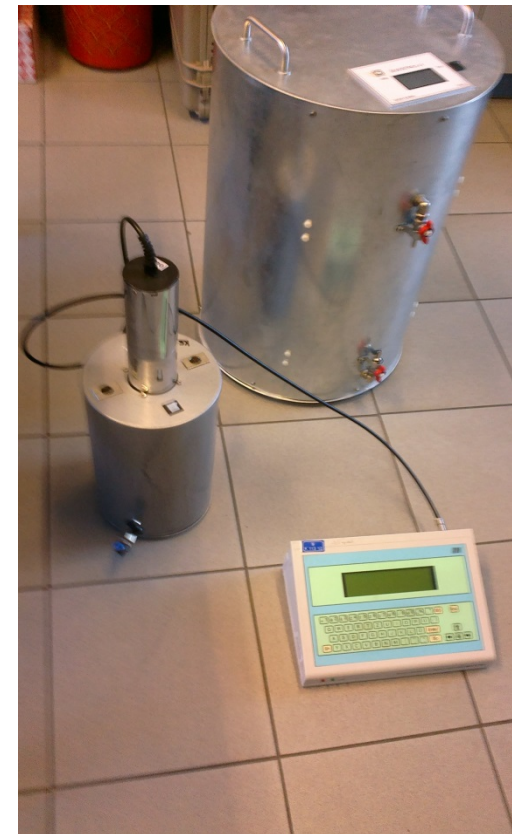
Fig.16 An example of measured radon outdoor daily variations and used radon low -level measurement instruments
