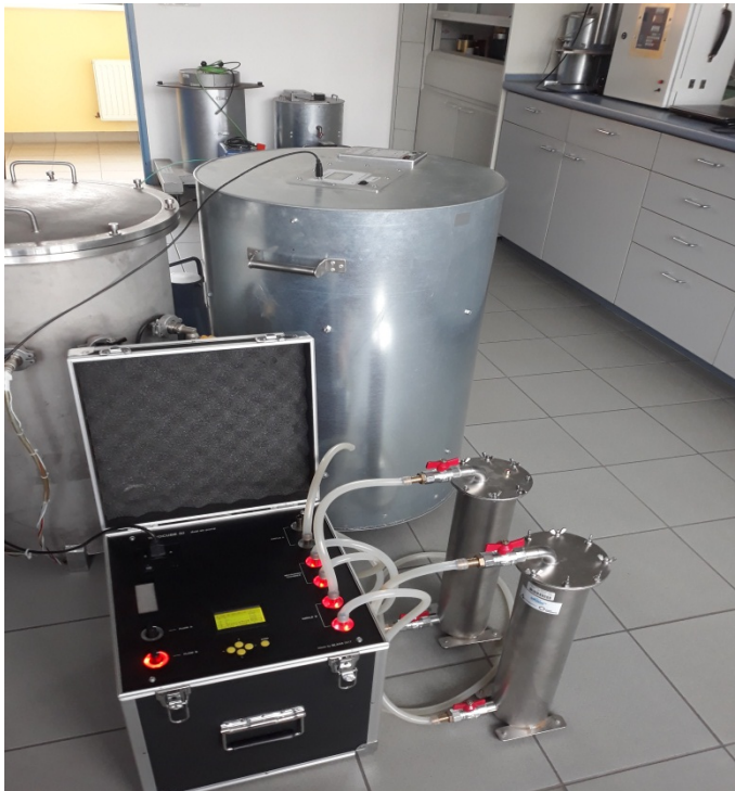
LLRM - 100 l ss -cylinder with 20 kV HV and alpha spectroscopy with powerful pump
