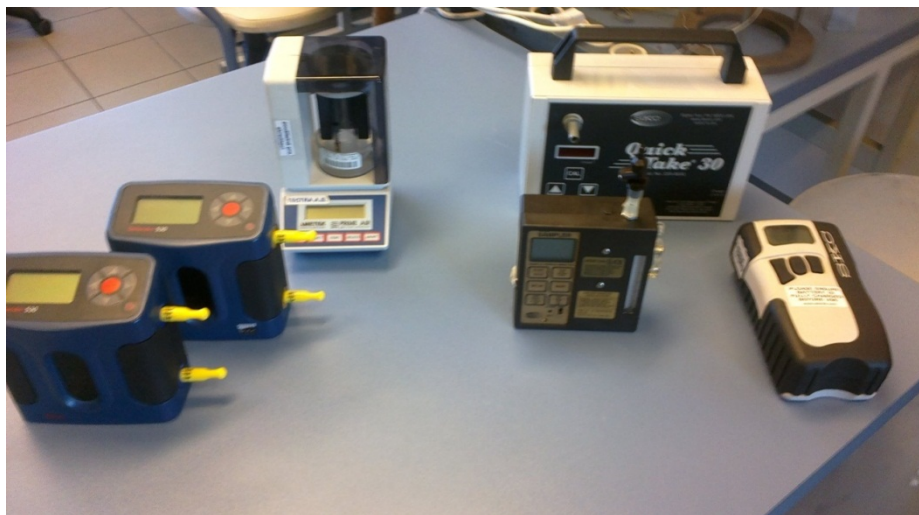
Fig. 5 Overview of used flow meter calibrators and pumps working in a wide rage.
