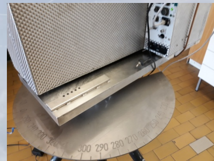
Final calibration for 1 IRIS pack 2 x 4 litre NaI(Tl) crystals
